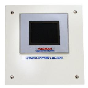
The System Controller offers many benefits to customers including, flexible scheduling of unit operations, scheduling unit rotation, setting system operating parameters, analyzing system performance and displaying alarms for YANMAR mCHP dealer trouble shooting accuracy and efficiency.
